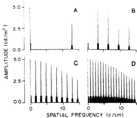
Fig. 2. The Fourier transforms of the profiles of Fig. 1. The mean luminance (0 cycles/cm) and the fundamental sinusoid (0.2 cycles/cm) are practically identical for the four conditions. What sampling does is to introduce a string of spurious high spatial frequencies at a repetition frequency determined by the sampling rate.
