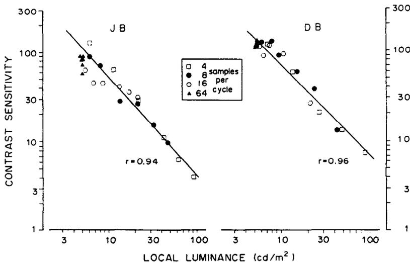
Fig. 7. Sensitivity for detection of a  $0.2\text{ c/deg}$  grating drifting at  $5\text{ Hz}$  ( $25\text{ deg/sec}$ ), plotted against the average local luminance of the sample bars. Measurements were made for the four sample frequencies, each mixed with 6 levels of veiling glare. Each point is the average of five measurements. The regression lines were fitted by least squares fit to the unaveraged data.
